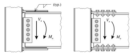
The shear can be carried by a single plate shear tab.
