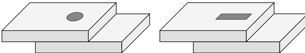
Both types of welds should be avoided due to the inherent low weld quality that results. It is often difficult to obtain adequate penetration of the weld due to limited access area at the bottom corners of the holes. In addition, it is difficult to avoid trapping slag and other inclusions as the weld pool rises in the hole.
