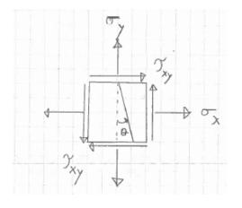
2) For Problem 3 & 4, Using the stress transformation equations, as discussed in class, write a computer program to solve for the principal stresses, the maximum and minimum shearing stresses, and their associated principal axes for a given state of stress. You may check your program by solving the problems given by McGraw-Hill Connect.
